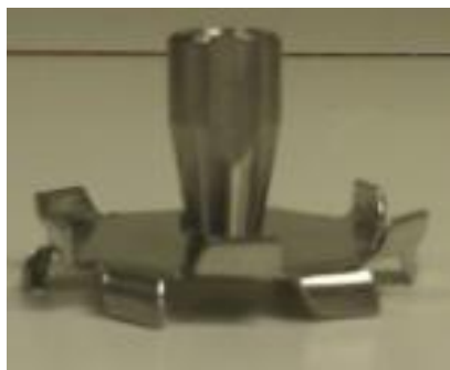
Figure 3. Dispersion impeller with a varying diameter ranging from 30-60 mm
